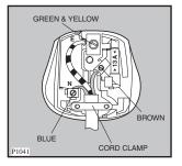
The wire coloured green and yellow must be connected to the terminal marked with the letter «E» or by the earth symbol = or coloured green and yellow.
